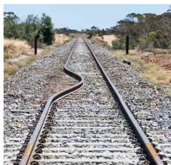
Fig 9.7 (a) Thermal expansion
