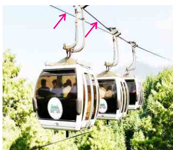
Fig 4.18 A chair lift hanging on supporting ropes.
